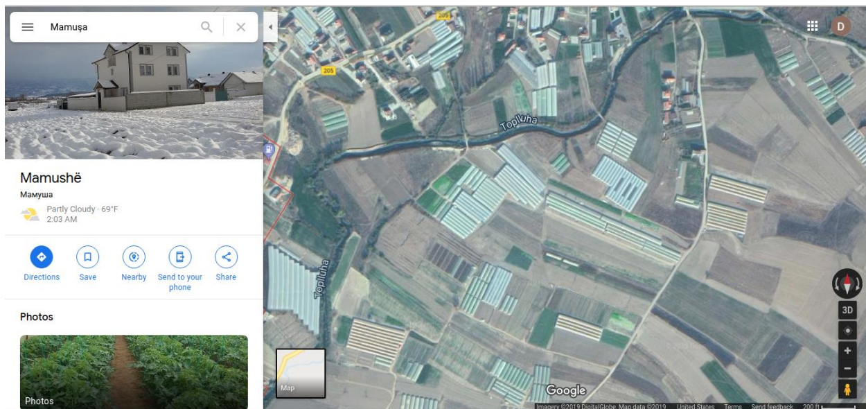
Figure 3: Overhead view from Google of Mamsuha. Greenhouses with numerous different orientations can be seen. Naturally ventilated greenhouses such as these should generally be oriented with the longest side perpendicular to the prevailing winds.
