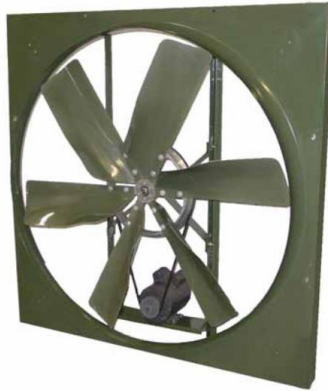
Figure 4: Exhaust fan for greenhouse. A 1,000 m 2 greenhouse would require seven to eight 48" diameter fans to exhaust air at one exchange per minute.
